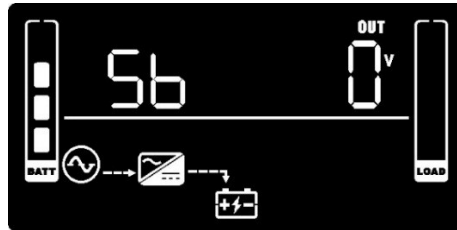
Figure 17: Display in standby mode
