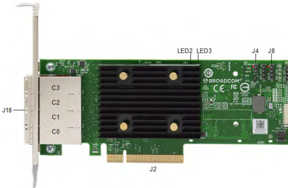
Figure 12: Card Layout of the HBA 9500-16e Storage Adapter
