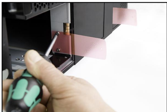
Figure 43. Transport Locking Screws Marked with Red Plastic Tab
