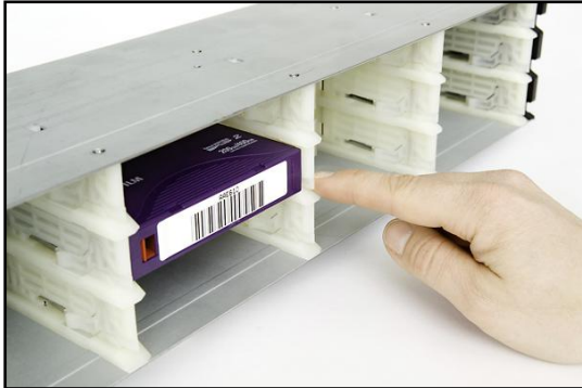
Figure 34. Ejecting a Cartridge from the Magazine Slot.
