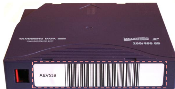
Figure 26. Positioning of Barcode Label for LTO Cartridges
