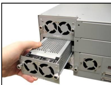
Figure 40. Hot-Swapping a Power Supply
