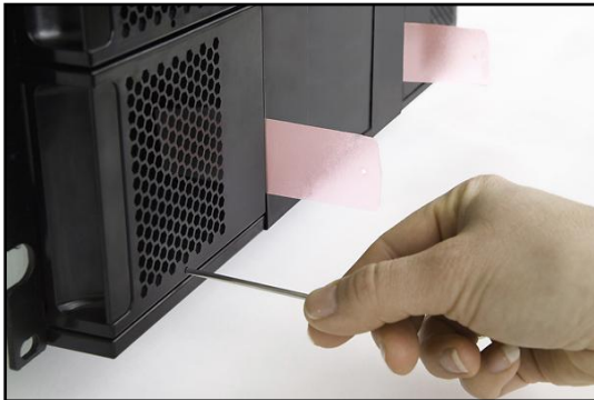
Figure 36. Ejecting a Magazine using the Emergency Release Tool
