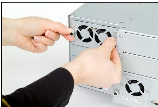
Figure 38. Replacing a Power Supply
