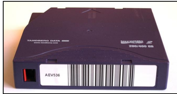
b) Write-enabled cartridge (The red write-protect switch slid to the left)
