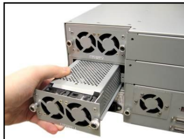
b) When inserting the power supply, keep it horizontally level to slide it in gently.
