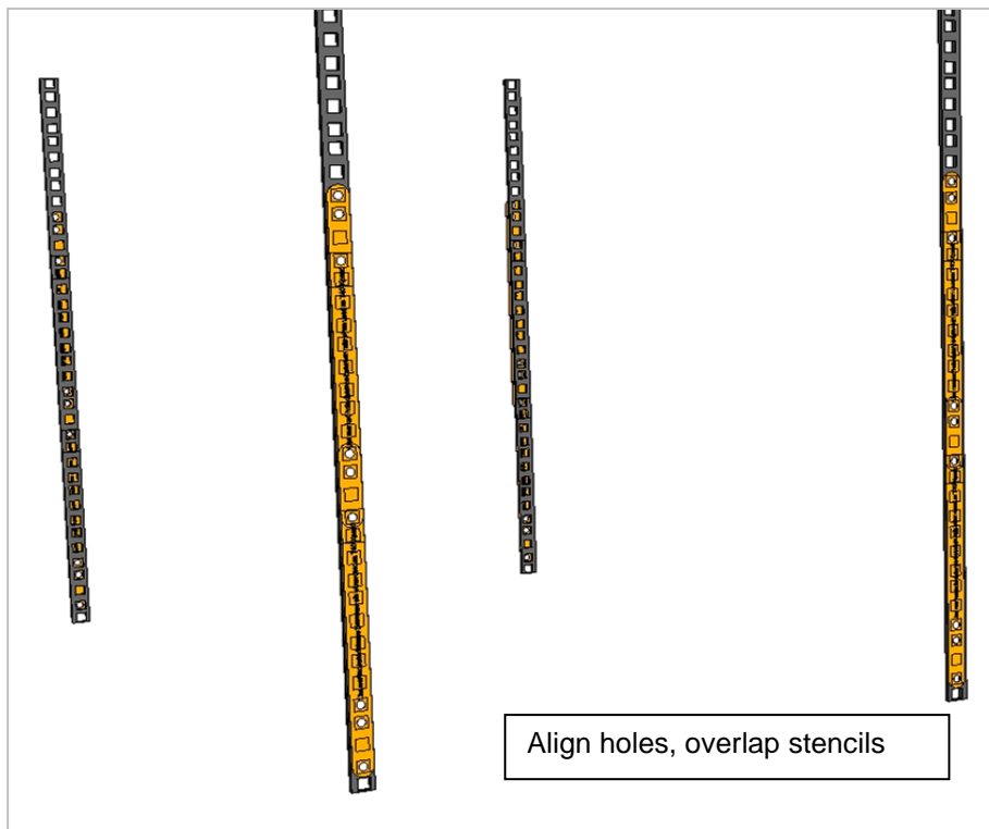
Figure 7. Aligning of the Rack Installation Stencils for systems with more than two units
