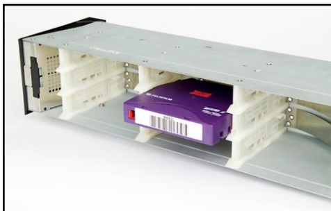
Figure 33. Inserting a Cartridge into the Magazine Slot
