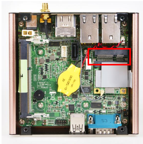
Locate the full-size MSATA slot on the board.
