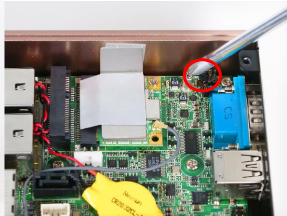
Remove the marked screw and use it to lock MSATA card to the slot in later installation.
