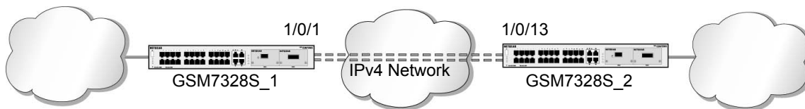
Figure 44. 6in4 tunnel between two switches
