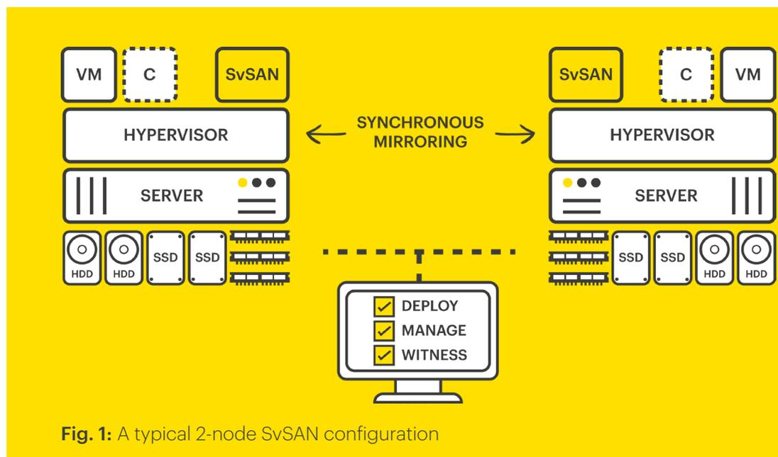
Fig. 1: A typical 2-node SvSAN configuration
