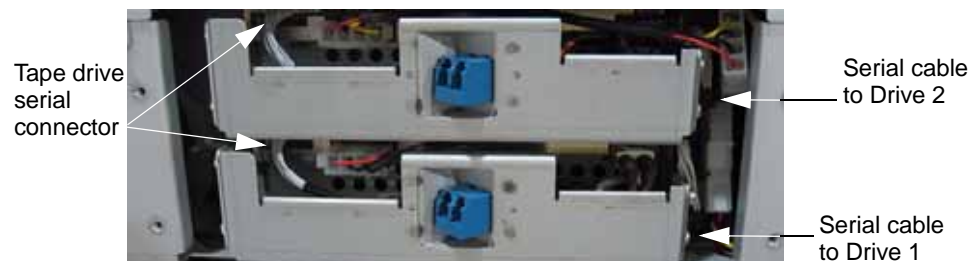
Figure F-2 Stowing the cables (LTO-4 tape drives pictured)
