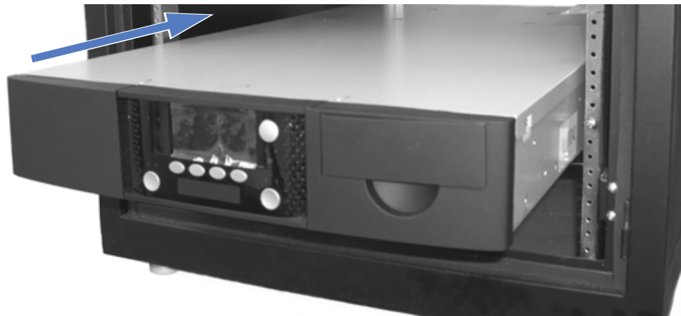
Figure 2-4 Placing the library on the rails
