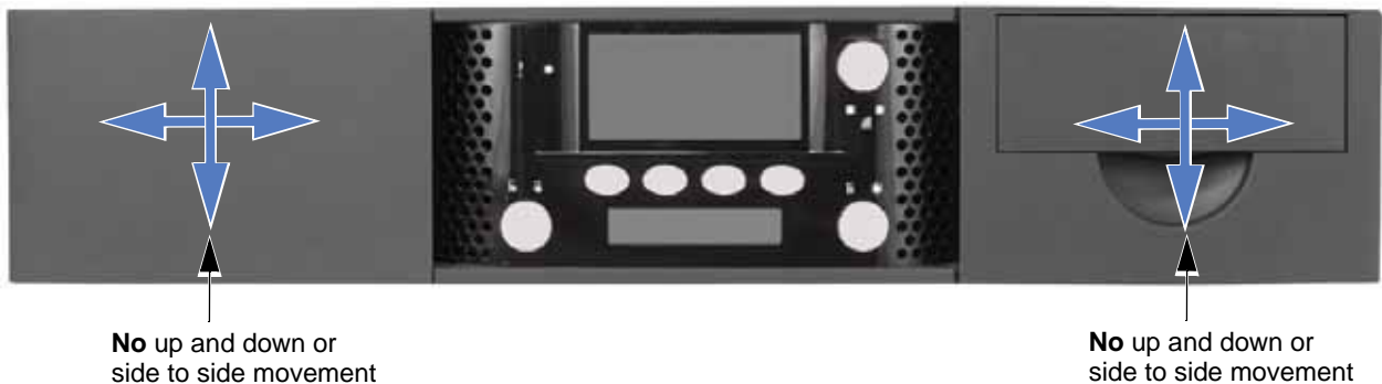
Figure 2-13 Shipping lock replacement preparation
