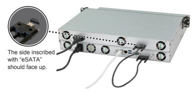
After the connection is complete, the expansion unit will be turned on or off automatically when the linked RackStation powers on or off.
