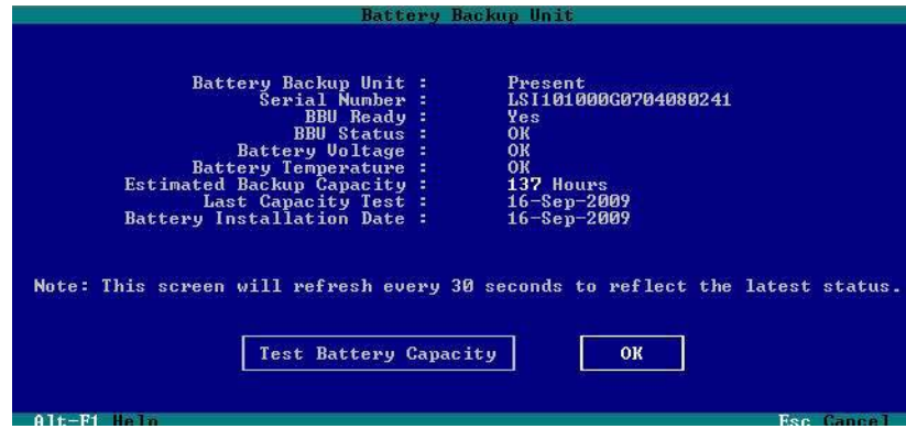
Figure 81. Battery Backup Information Screen in 3BM
