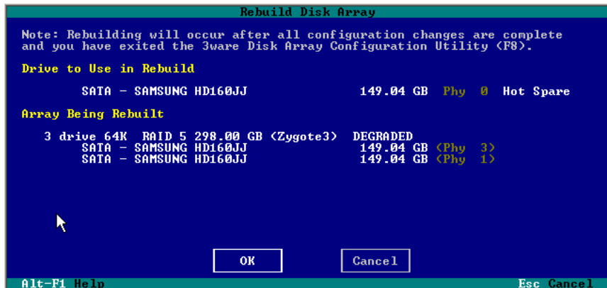
Figure 71. Rebuild Disk Array Screen
