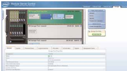
Create storage pools (either non-virtualized or virtualized) and virtual drives, and map virtual drives to multiple servers using the Intel Modular Server Virtualization Manager and Intel Shared LUN features
