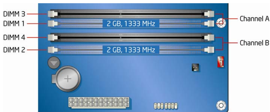
Figure 12. Example Dual Channel Memory Configuration with Two DIMMs
