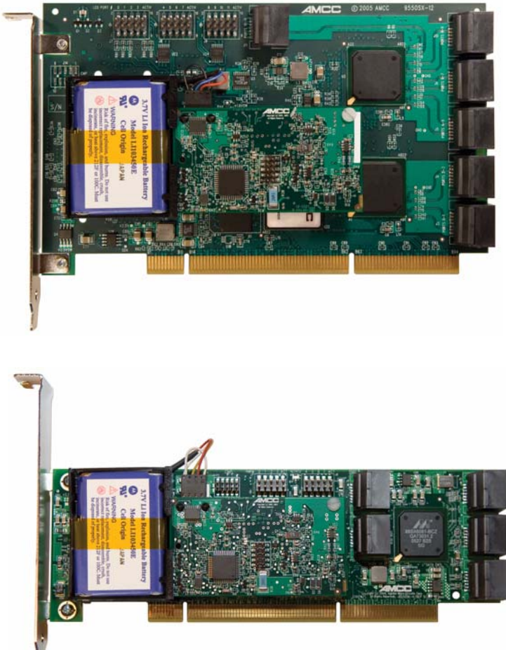
Figure 30. BBU installed on controllers
