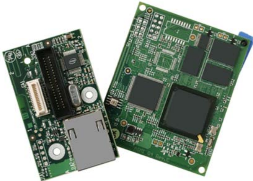
Figure 2. Intel® Remote Management Module 2 and NIC
