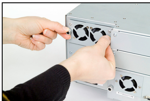
Figure 37. Replacing a Power Supply
