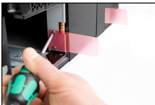
Figure 21. Transport Locking Screws Marked with Red Plastic Tabs
