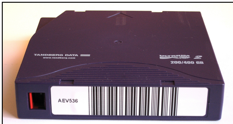
Figure 26. Positioning of Barcode Label for LTO Cartridges
