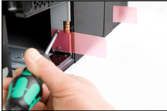
Figure 42. Transport Locking Screws Marked with Red Plastic Tab
