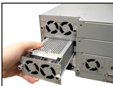
b) When inserting the power supply, keep it horizontally level to slide it in gently.
