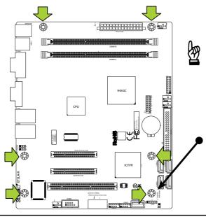
Important: If the chassis does not provide mounting support at this location, please install a plastic standoff support, similar to the illustration below. There are two pieces provided in your package.
