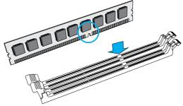
Push the Lock/Release tabs to their Release positions. Make sure that the DIMM module's side notches align with the slot's Lock/Release tabs as it is pressed in.
