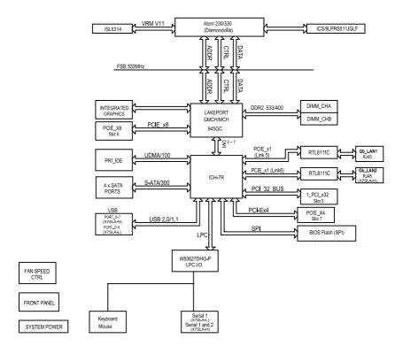
X7SLA-L / X7SLA-H Block Diagram
