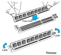
When the module is properlly inserted, the Lock/Release tabs will automatically secure the DIMM module, locking it into place.
