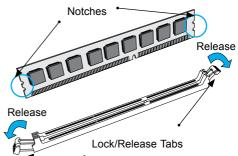
Insert the DIMM module vertically and press down until the module snaps into place.
