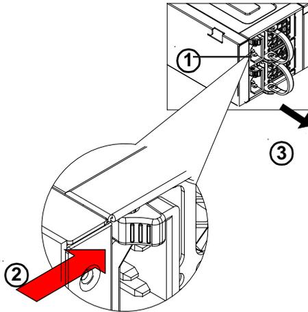
3. Once the power supply module is released from its locking position, remove it from the chassis.
