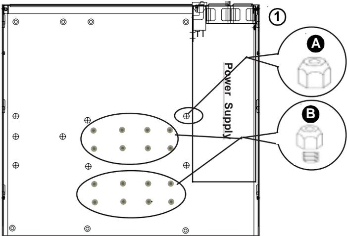
2. On the chassis, install standoffs in the mounting holes that are corresponding to the mounting holes on the motherboard.
