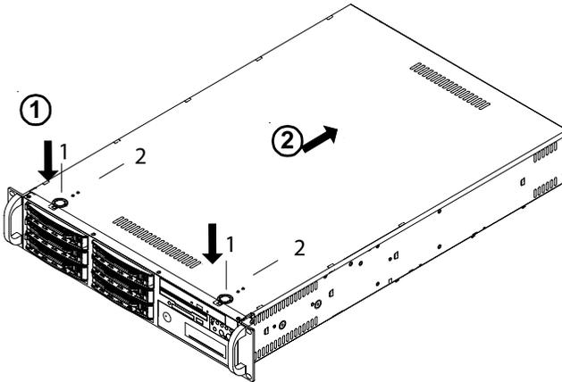
2. Once the top cover is released from its locking position, push the cover toward the rear side and slide it out from the chassis.
