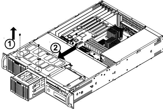
3. Remove the screws to loosen the drive tray. Once loosened, pull it out from its housing. Then, mount a hard drive in the drive tray and secure it with screws as shown below.
