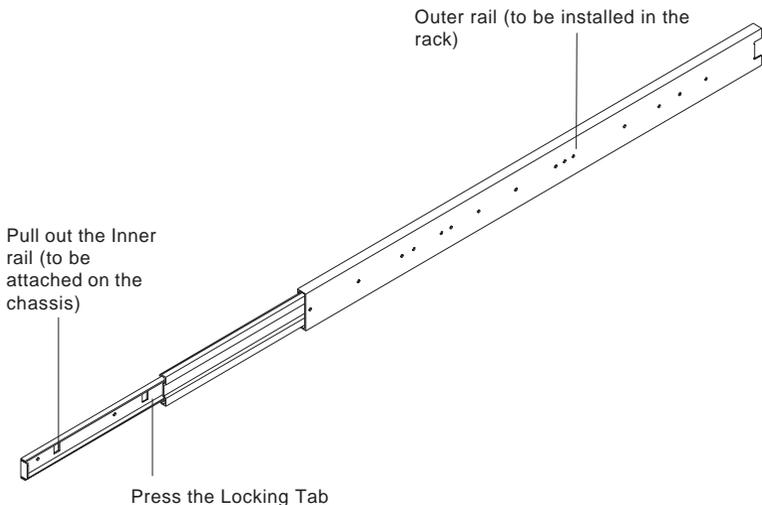
3. Locate the five rail hooks on each side of the chassis and the five corresponding holes on each of the inner rail.
