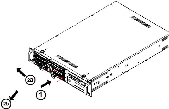
3. Remove the screws to loosen the drive tray. Once loosened, pull it out from its housing. Then, mount a hard drive in the drive tray and secure it with screws as shown below.
