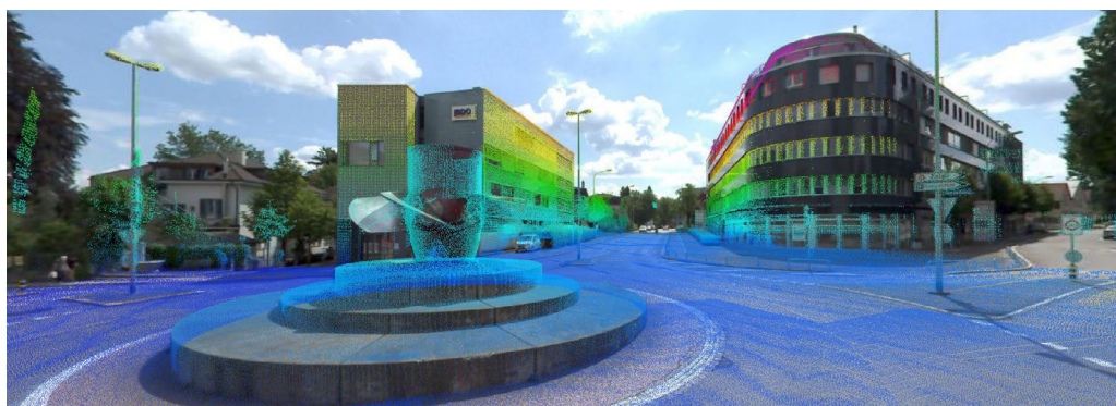
The assessment produces three-dimensional 360-degree images of the entire road space. These are the basis for digital terrain models.
