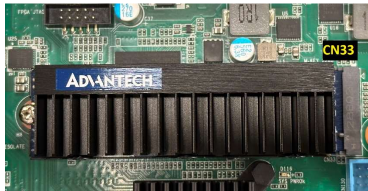
Figure 3-8 M.2 M-KEY SATA/NVMe SSD Installation
