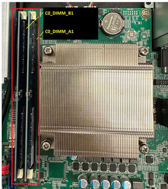
Figure 3.2-5 DRAM Installation Order
