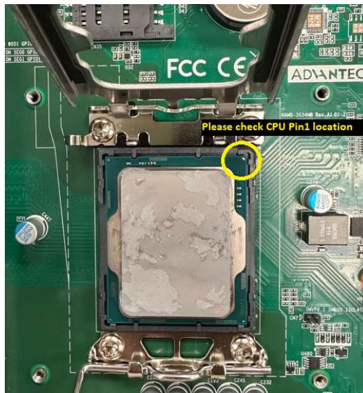
Figure 3-5 CPU Installation – install CPU and check Pin1 location
