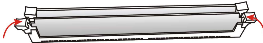
Figure 3-38: Seating the DIMM in the Socket
