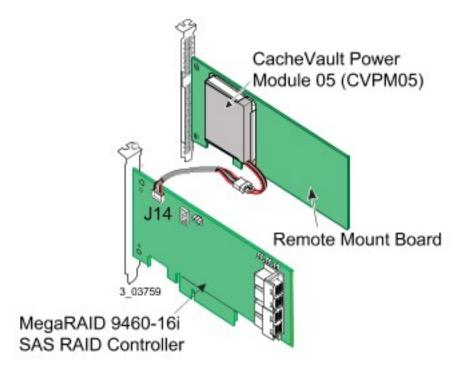
4. Insert the other 9-pin cable connector into the 9-pin connector on the remote CVPM05 module. Align the cable connectors to make sure they are connected correctly.
