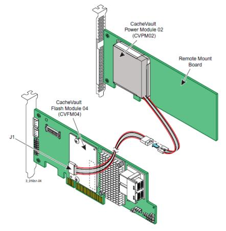
4. Insert the other 9-pin cable connector into the 9-pin connector on the remote CVPM02 module. Align the cable connectors to make sure they are connected correctly.
