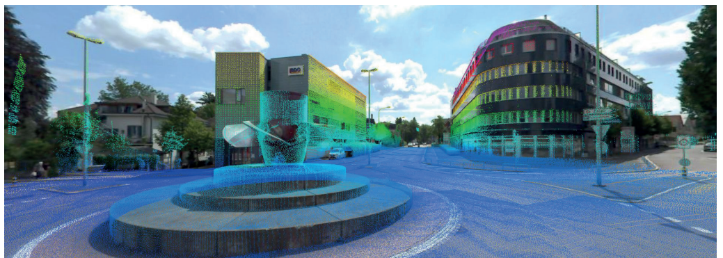
The assessment produces three-dimensional 360-degree images of the entire road space. These are the basis for digital terrain models.
