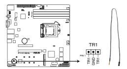
P11C-M/4L Thermal sensor cable connector
