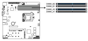
P11C-M/4L 288-pin DDR4 DIMM sockets
