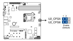
P11C-M/4L CPU PCIE CFG setting
