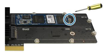
**d** Repeat previous three steps if installing another M.2 SSD is needed. Slots are numbered as shown below.
