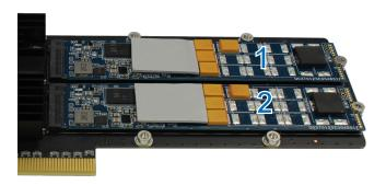
**e** Tighten the heatsink with four screws. Please make sure the heatsink is firmly attached to the adapter card to ensure the smooth running of the M.2 SSD.
