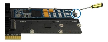
**c** Remove the protective film from the thermal pad and attach the thermal pad to the controller of SNV3500-400G. Attach the rubber next to the screw pillar.
