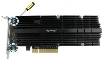
**b** Tighten the full-height bracket with two screws.
