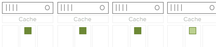
Figure 44. RAID-5 erasure coding
