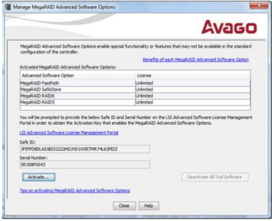
Figure 234 Manage MegaRAID Advanced Software Options Dialog
