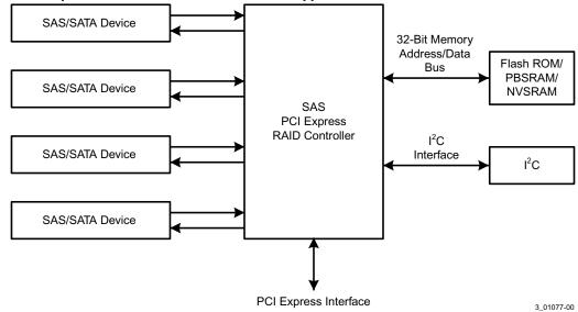
The following figure shows an example of a SAS RAID controller configured with an LSISASx12 expander that is connected to SAS disks, SATA II disks, or both.
