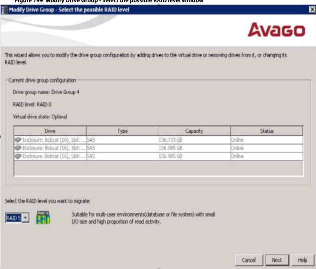
Figure 199 Modify Drive Group - Select the possible RAID level Window
