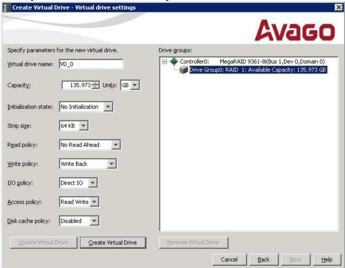
Figure 187 Create Virtual Drive - Virtual drive settings Window
