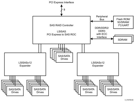
Figure 2 Example of an Broadcom SAS RAID Controller Configured with an LSISASx12 Expander
