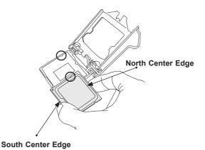
Align the CPU key that is the semi-circle cutouts against the socket keys. Once it is aligned, carefully lower the CPU straight down into the socket. (Do not drop the CPU on the socket. Do not move the CPU horizontally or vertically.
