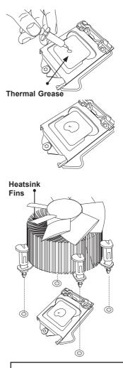
Recommended Supermicro heatsink: SNK-P0046A4 active heatsink
