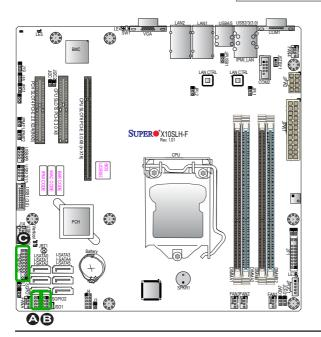
A.T-SGPIO 1 B.T-SGPIO 2 C.JTPM1
