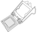
Do not rub the CPU against the surface or against any pins of the socket to avoid damaging the CPU or the socket.)
