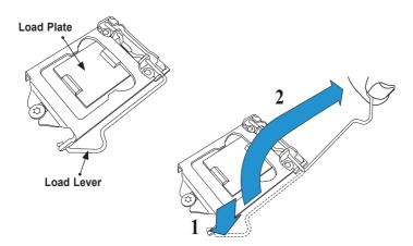
2. Gently lift the load lever to open the load plate. Remove the plastic cap.
