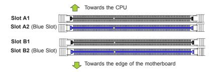
The X10SLH-F supports up to 32GB of Unbuffered (UDIMM) DDR3 ECC 1600/1333 MHz (1.35V/1.5V) memory in 4 slots. Populating these DIMM modules with a pair of memory modules of the same type and same size will result in interleaved memory, which will improve memory performance. Please refer to the table below:
