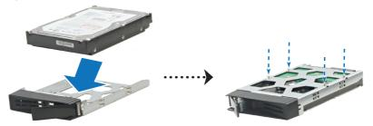
For 2.5" Hard Disk: Place the hard disk in the rectangular area (shown below) of the hard drive tray, turn the tray upside down, and then tighten the screws to secure the hard disk.
