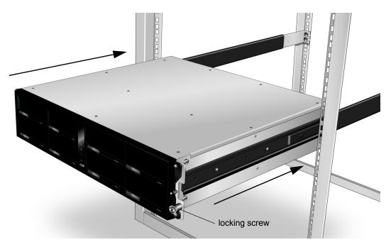
! Important Do not place anything on top of the rackmounted unit when it is extended from the rack.
