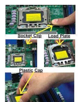
Hold the north & south edges of the plastic cap to remove it
