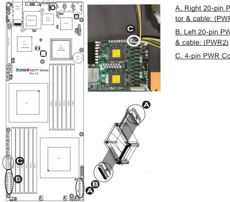
A. Right 20-pin PWR connector & cable: (PWR1) B. Left 20-pin PWR connector
