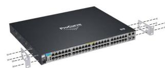
Mount the switch and connect the power cord.
