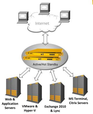
The LM2600 can load balance up to 1000 servers and 500 virtual clusters
