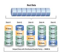
**RAID 6:** Two sets of parity data, P + Q, are striped across disks. RAID 6 safeguards against data loss during rebuild mode by allowing up to two consecutive drive failures for maximum fault tolerance.
