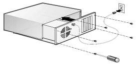
**3** Locate an unused 64-bit PCI/PCI-X expansion slot and remove the expansion slot cover. If the computer does not have a 64-bit slot, you can install the card in a 32-bit PCI slot. The Adaptec SCSI Card 29320A supports both 5V and 3.3V 64-bit slots. (The expansion slot must be compliant with PCI Rev. 2.1 or PCI-X Rev. 1.0 and must support Bus Mastering.) Save the slot cover screw for use in Step 4.
