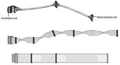
**2** Plug the nonterminated end of the cable(s) to the internal LVD connector.
