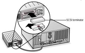
Connect the other external SCSI devices by linking each device to the previous one, as shown below. Terminate only the device at the end of the chain.
