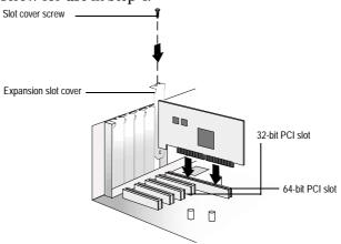
Computers may have vertical or horizontal expansion slots. Refer to your computer manual to locate the PCI/PCI-X slots. If your computer is a tower model, lay it on its side to allow for easier installation of the Adaptec SCSI Card 29320A.
