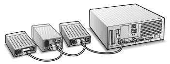
**4** Connect power cables to all external device(s) and to the computer.
