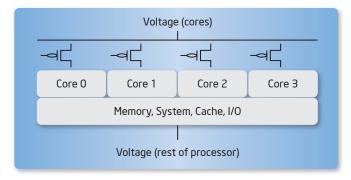
**Figure 3.** Integrated Power Gates enable idle cores to go to near-zero power independently.
