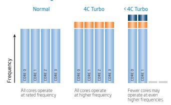
**Figure 1.** Intel® Turbo Boost Technology increases performance by increasing processor frequency and enabling faster speeds when conditions allow.
