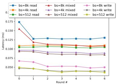
The Steady State Convergence Plot shows the mean latency for all block sizes of random read, mixed workload and write.
