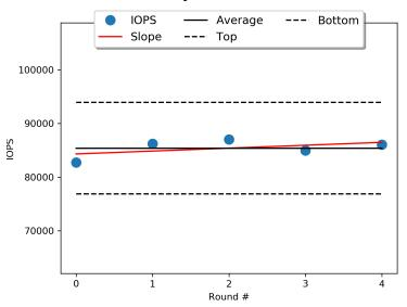
The Steady State Verification Plot shows the measured IOPS of 4k random writes, the 20% average window and the slope of the linear best fit line in the measurement window.
