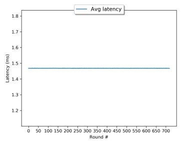
The Write Saturation Latency Plot shows the mean latency of 4k random writes over all rounds.
