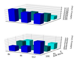
The Latency Measurement 3D Plot shows the average latency on top and the max latency below it. For the measurement window every workload including all block sizes is plotted.
