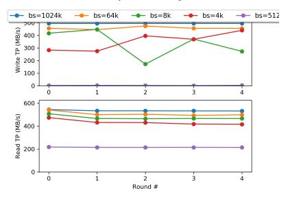
The Read/Write Steady State Convergence Plot shows the bandwidth for all block sizes of seq. reads over all rounds. On the top the write throughput is plotted, below the throughput for read.
