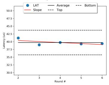
The Steady State Verification Plot shows the mean latency of 4k random writes, the 20% average window and the slope of the linear best fit line in the measurement window.
