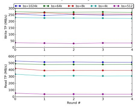
The Read/Write Steady State Convergence Plot shows the bandwidth for all block sizes of seq. reads over all rounds. On the top the write throughput is plotted, below the throughput for read.
