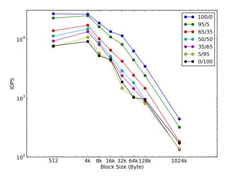
The Measurement Plot shows the average of IOPS in the measurement window. For every workload the IOPS of all block sizes are plotted.
