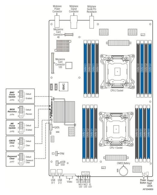
Figure 9. Recovery Jumper Blocks
