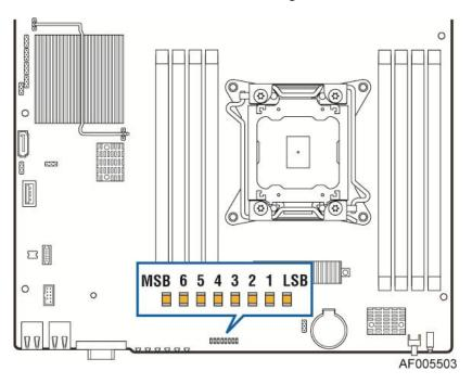
Figure 10. POST Code Diagnostic LED Decoder
