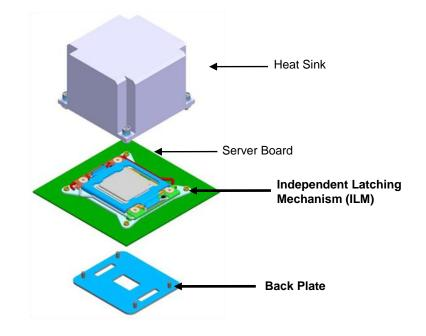
Figure 4. Processor Socket Assembly
