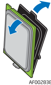
Figure 23. Removing Protective Shipping Cover
