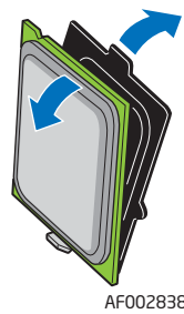
Figure 13. Removing the Processor Protective Cover
